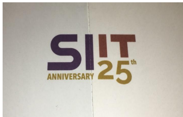
Fig. 3 Digital photograph of PEDOT:PSS film coated onto the glass substrate showing its high visible transparency
