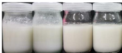
Fig.3 The resulting W_1/O/W_2 double emulsions with 700ppmCS/500ppmCMC, 700ppmCS/700ppmCMC, 700ppmCS/100ppmLS and 700ppmCS/200ppmLS complex stabilizer, respectively
