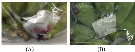
Fig. 4 Photos of the sachets inside the banana packaging during the storage for 7 days; (A) uncoated sachet inside banana packaging; (B) wax-coated hydrophobic sachet inside the banana packaging
