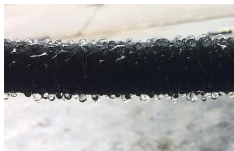
Figure 1 Porous pipe made from GRT mixed NR/RR
